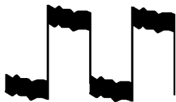
Typical peak detect display
