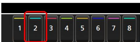
The selected channel is added to the Waveform View and a Channel badge is added to the Settings bar.
