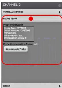
3. Tap the **Other** panel to set probe deskew, external attenuation, and alternate units parameters.
