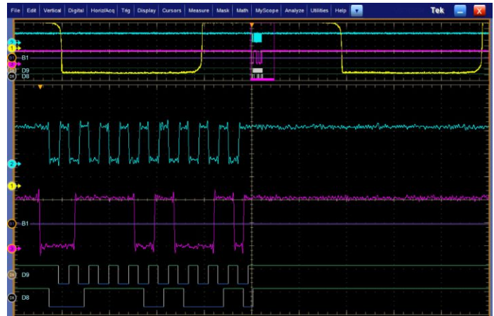
Integrated Logic Channels – Provide time-correlated analog and digital visibility for system debugging.
