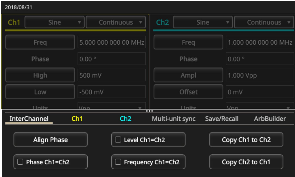
Figure 44: Align Phase CH1 and CH2
