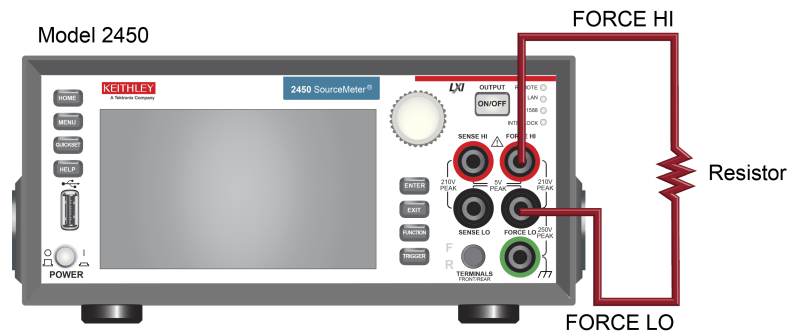
Figure 15: Model 2450 2-wire front-panel connections
