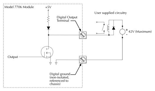
Figure 14 **Typical digital output (no external power supply)**
