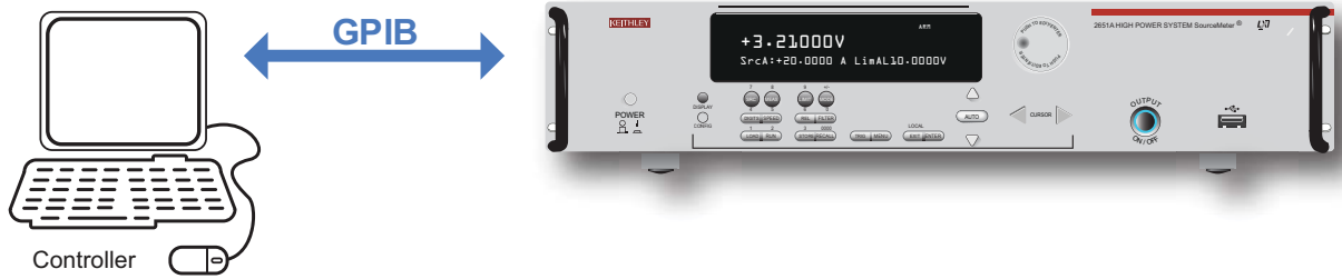
Figure 12: GPIB communication example for fast ADC
