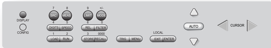
Figure 2: Setup and control keys
