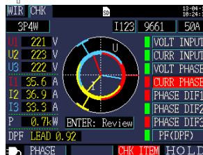
Wiring Check screen
