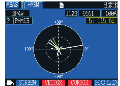
Harmonic power phase angle graph screen
