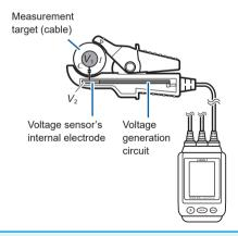
$V_2$  is controlled so that I = 0. Assuming that  $V_1 = V_2$  when I = 0,  $V_2$  is measured. Based on equation (1), I = 0 when V = 0 (when the measurement target and the voltage sensor's internal electrode have the same potential).
