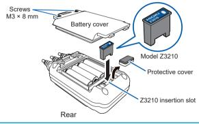
To maintain the dust resistance and water resistance, put the protective cover on the Z3210 insertion slot regardless of the presence or absence of the Z3210.
