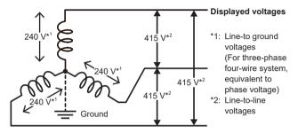
The 400 V line depicted in the figure has line-to-line voltages each of which is 415 V yet has line-to-ground voltages each of which is approximately 240 V. You can use a measuring instrument whose the input rating of a line-to-ground voltage is 300 V to measure this circuit
