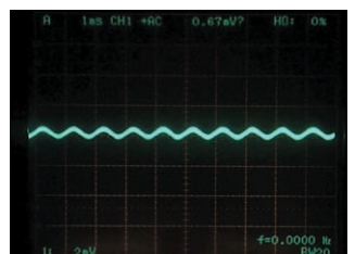
Input: 1 kHz sine wave 50 mAp-p (Oscilloscope bandwidth 20 MHz)
