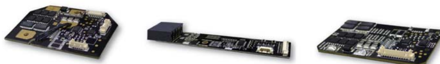
BMS test board
