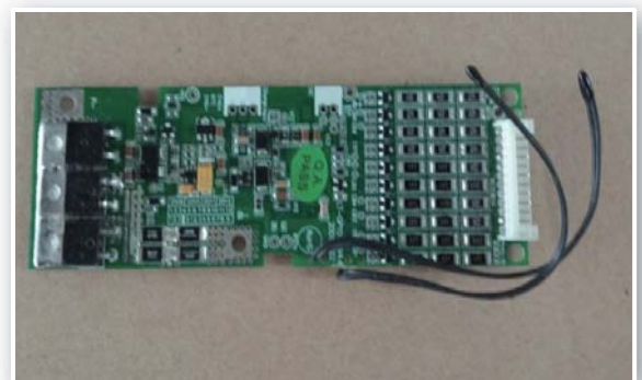
BMS test board
