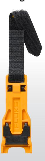
The TLPV-UTOOL is designed to quickly disconnect solar PV connectors. It works with Fluke TLPV1 and TLPV2 Test Leads that have Staubli MC4 connectors. The tool's unique hinge design allows for unlocking in both parallel and perpendicular configurations, providing versatility in various installation scenarios. Backed by a 90-day warranty, the TLPV-UTOOL ensures reliable performance and ease of use for professionals in the solar industry.
