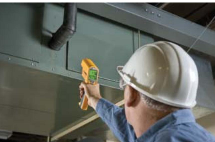
When compared with contact thermometers, time savings can be measured in hundreds of man-hours annually, and technicians can do a more thorough job because the speed and ease of operation of a Fluke non-contact thermometer allows more frequent gathering of temperature data.
