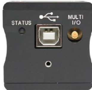
Figure 2.1 USB Connector and Status LED
