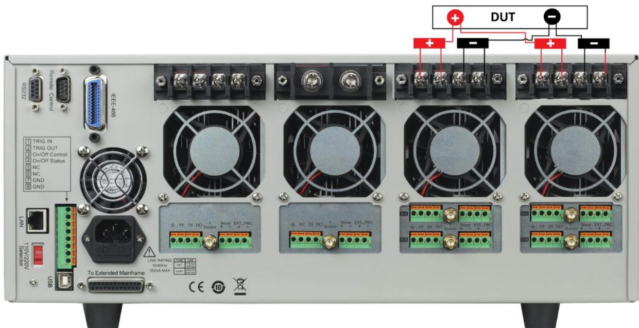
Figure 3.2 Parallel Module Connection
