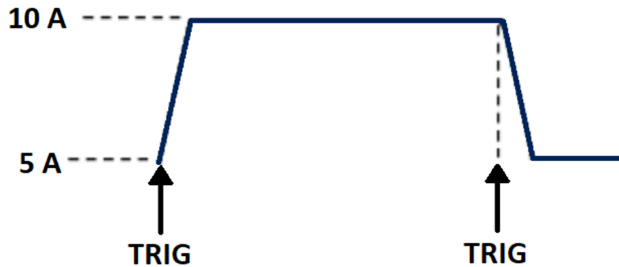
Figure 4.12 Toggle Transient Operation
