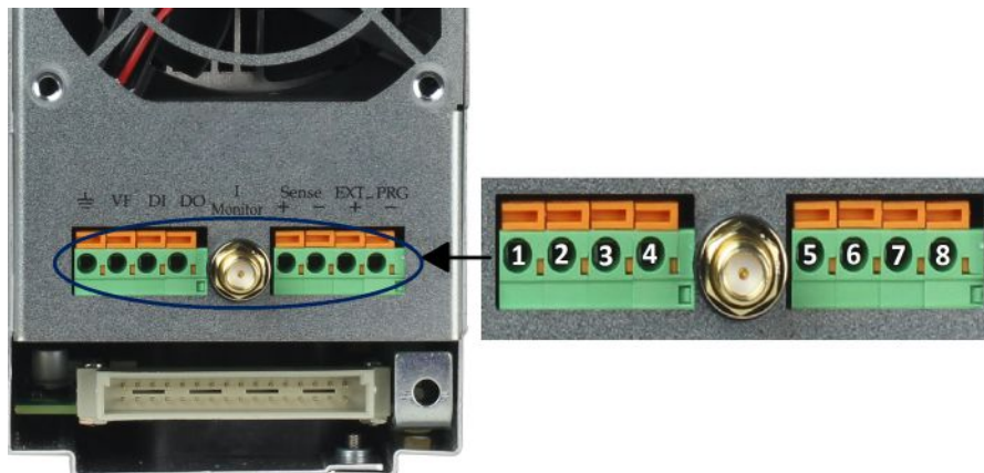
Figure 4.16 Single-Channel Control Module Link
