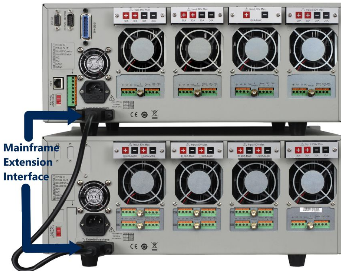
Figure 3.5 Mainframe Extension Connection
