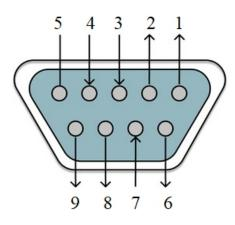
Figure 5.6 RS232 Pinout
