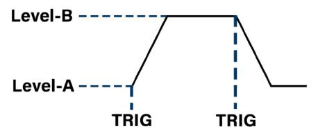
Figure 4.8 Toggle Transient Operation
