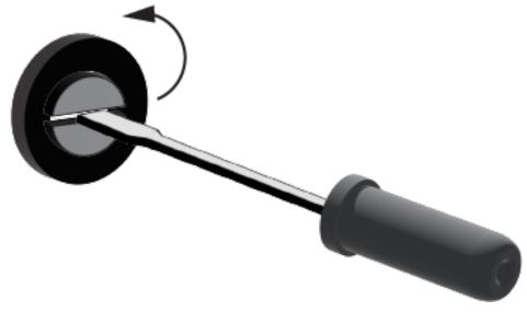
Figure 2.1 Fuse Removal
