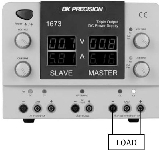
Figure 6 – Parallel Tracking Mode Load Connection
