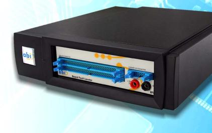
In and out of circuit • Through hole or SMT • NAND gates to CPUs • DIL, PLCC or SOIC . Standard and custom logic • TTL or CMOS •
