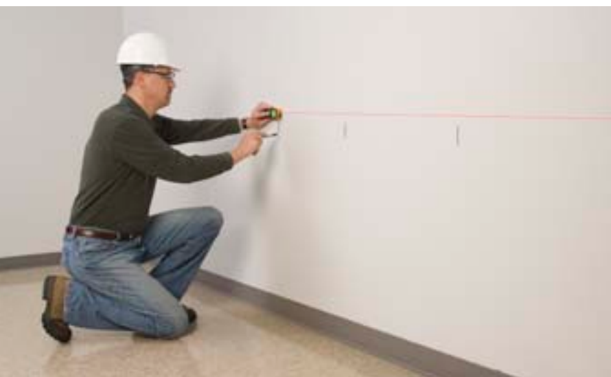
Incremental measurements using the stakeout feature (421D only).
